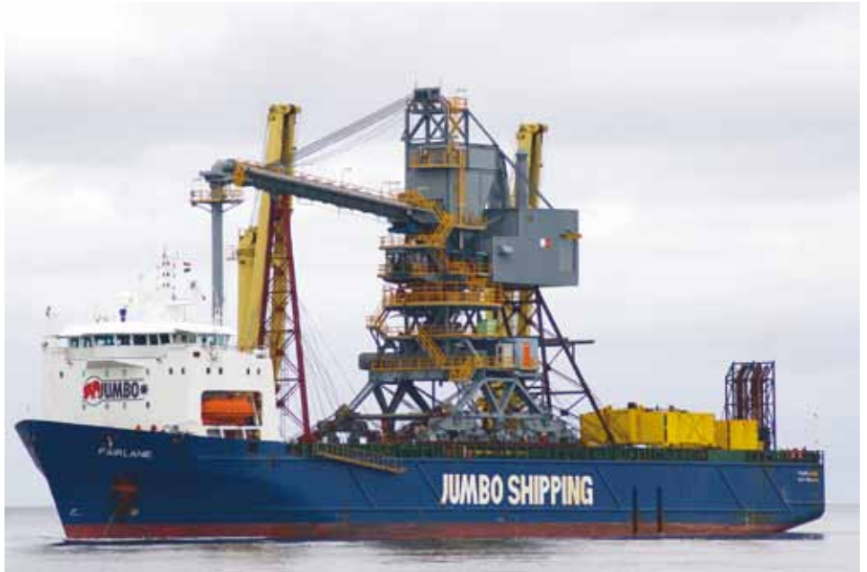
A new ship unloader arrives in Bluff in August 2011 for the Tiwai aluminium smelter. The unloader will replace the previous one which discharges at 230 tonnes – the replacement is capable of 1000 tonnes (photo by Harry Holland)
